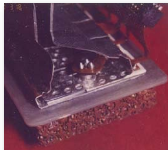
½ Bridge 50 kW Module, 4 in 3 Integral RMF HX on Cu Metalized AlN base, q=1 kW/in 2 , liquid cooled
