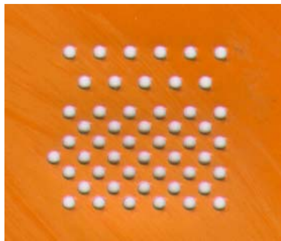
Punched or laser processed through vias
